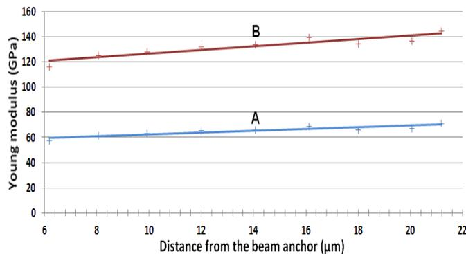
Fig. 11. Extraction of the beam young modulus. A) based on design dimensions. B) based on measured dimensions.
