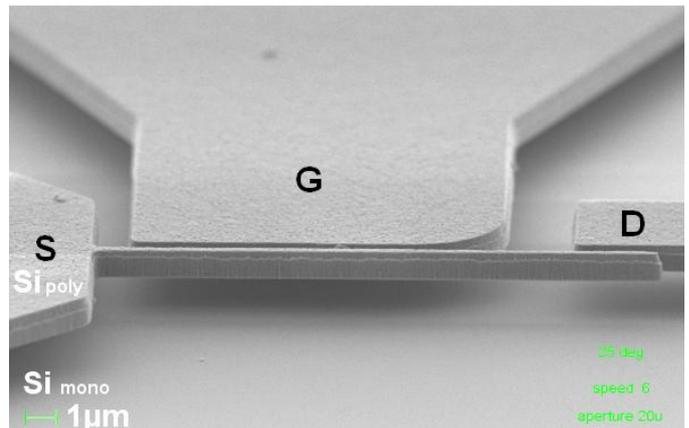
Fig. 2. Scanning Electron Microscopy image of a NS.
