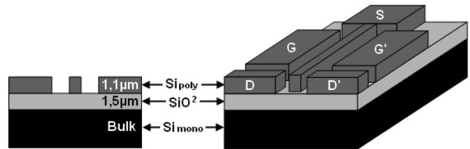
Fig. 1. Structure of a NS. (Source (S), Gate (G), Drain (D)). Beam: 300nm width, 1100 nm thick and 20  $\mu\text{m}$  length.
