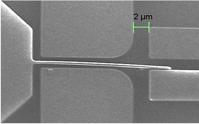
Fig. 4. SEM image of a NS at the ON state.
