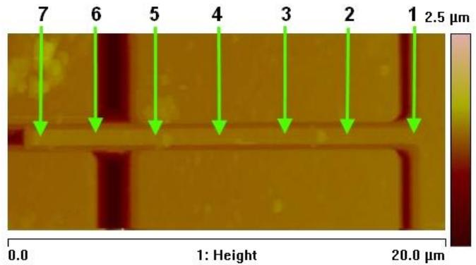
Fig. 8. AFM image of a NS with the position of approach-retract curves.
