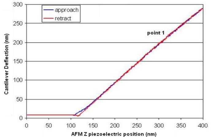
Fig. 9. Approach-retract curve at point 1 (cf. Fig. 8).
