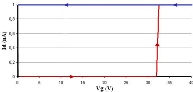
Fig. 6. Experimental electrical characterization of a NS. The beam staying stuck to the drain after ON state, as shown in Fig. 4. Measurement parameters:  $V_S=0V$ ,  $V_D=3V$ , compliance 1nA.
