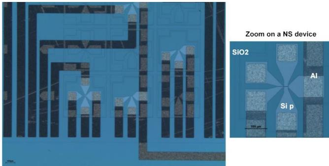
Fig. 13. Optical image of the improved design with electrical contacts routed to the edge of the chip.
