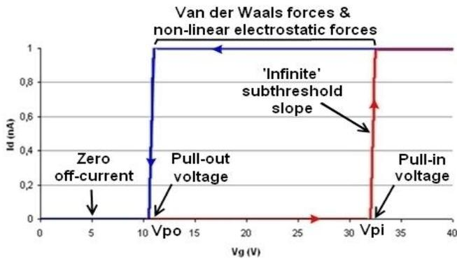
Fig. 5. Experimental electrical characterization of a NS. Measurement parameters:  $V_S=0V$ ,  $V_D=3V$ , compliance 1nA.
