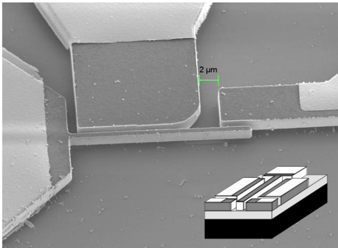
Fig. 14. SEM image showing thin platinum layer coating on the NS side walls to improve the device structure.
