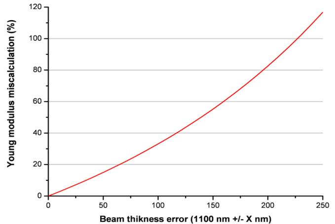
Fig. 12. Young modulus miscalculation depending of the beam thickness error.
