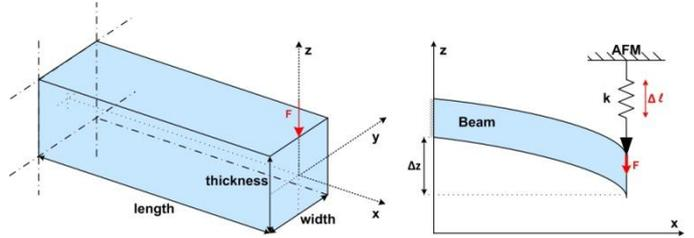
Fig. 7. Schematic of the young modulus extraction model.
