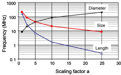
Figure 1. Effect of the reduction of size on the resonance frequency of a cantilever. The reference device ( $\alpha=1$ ) is a 50 nm wide, 1  $\mu\text{m}$  long NW.
