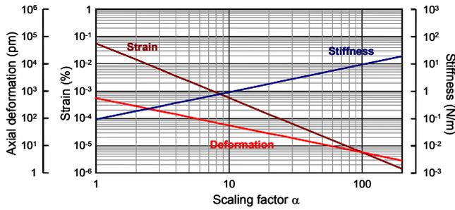
Figure 4. Effect of the size scaling down of a cantilever in terms of axial strain, axial deformation and stiffness under fixed force (80nN).
