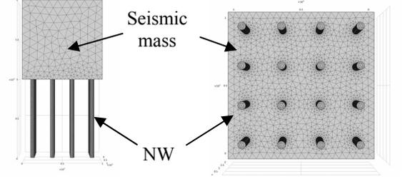
Figure 2. Side view and top view of the elementary cell simulated to calculate the resonance frequency of an array of vertical NWs connected by a seismic mass. The NWs are considered as fully clamped to a solid substrate at their bottom. The seismic mass is supposed to be made of tungsten.
