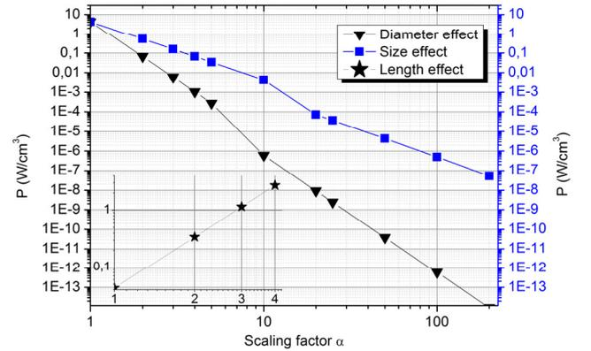
Figure 5. Power density of a mechanical energy harvesting device based on vertically integrated ZnO NWs. Effect of diameter and size scaling down (main graph) and of length scaling down (inset), with a constant force equal to 10nN or 1nN, respectively.
