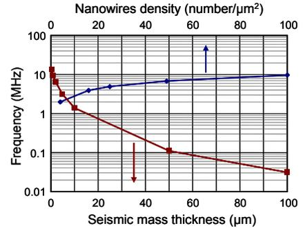
Figure 3. Resonance frequency of the structure as a function of (a) thickness of the seismic mass and (b) number of NWs per  $\mu\text{m}^2$ .
